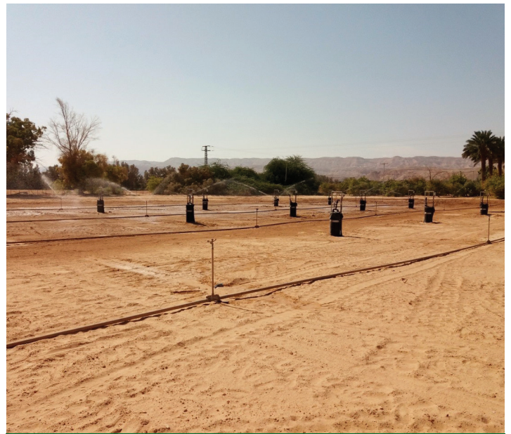
Figure 2: Soil surface of the lysimeter before planting the trees
